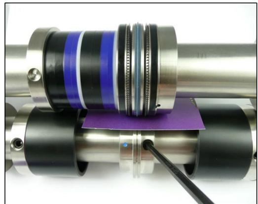
Now, while the sheet is still between the male and female, tighten the set screw on the female. It should be locked into a centered position. You can run a sheet to check this. If it's centered correctly, you'll have a smooth, rounded bead on the inside of the fold.
